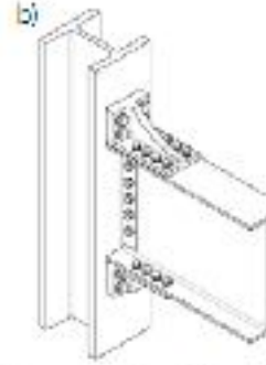
Figure 6: Kaiser bolted bracket (KBB) connection (a) welded and (b) bolted to the beam.
