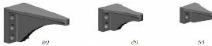
Kaiser bolted bracket W-series configurations: (a) six column bolts, W-3; (b) four column bolts, W-2 and W-1; and (c) four column bolts, W-2 and W-1.
